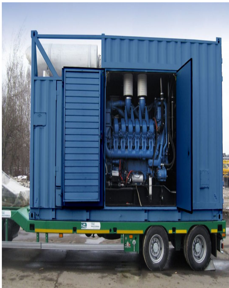
photo of a mobile diesel generator
