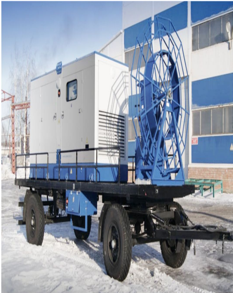
photo of a mobile diesel generator
