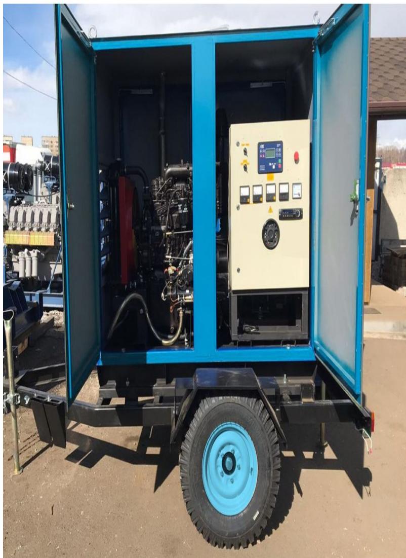
photo of a mobile diesel generator (on chassis)
