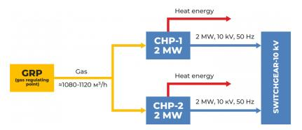
The points of connection of the gas piston plant to the existing power supply system of the enterprise are specified at the stage of design work and depend on the existing scheme of electricity, heat and gas supply of the enterprise.
