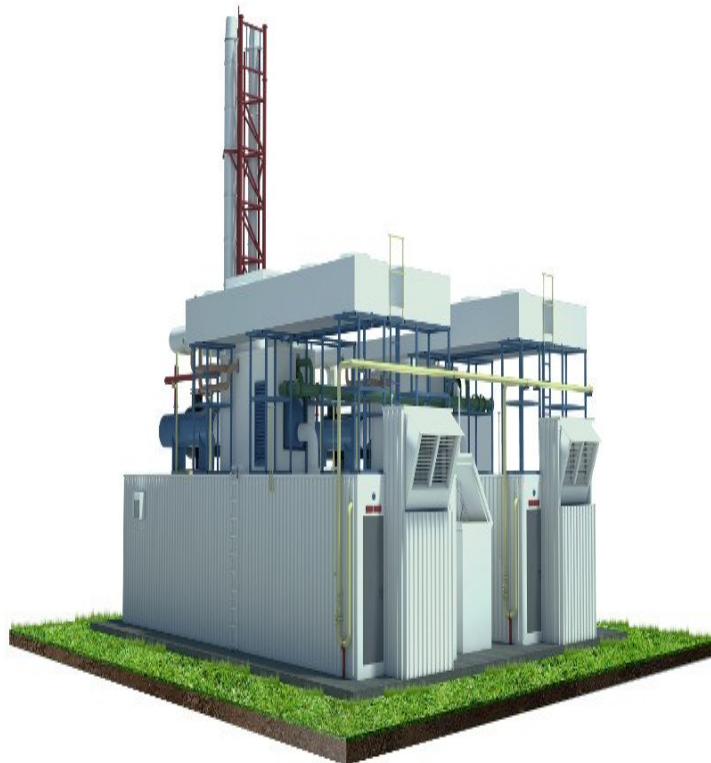
A 3D model of a mini-thermal power plant in a block-modular design
